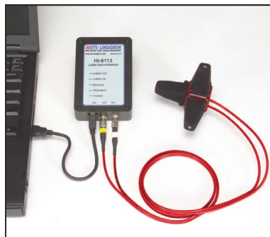
A USB port supplies power for the laser.
