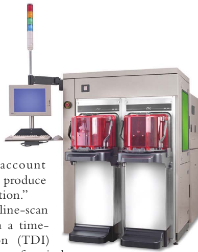
FIGURE 2. The WS-3000 system inspects 200- and 300-mm wafers. This unit combines 3-D laser technology with a 2-D high-resolution camera to provide quantitative and qualitative inspection information.
