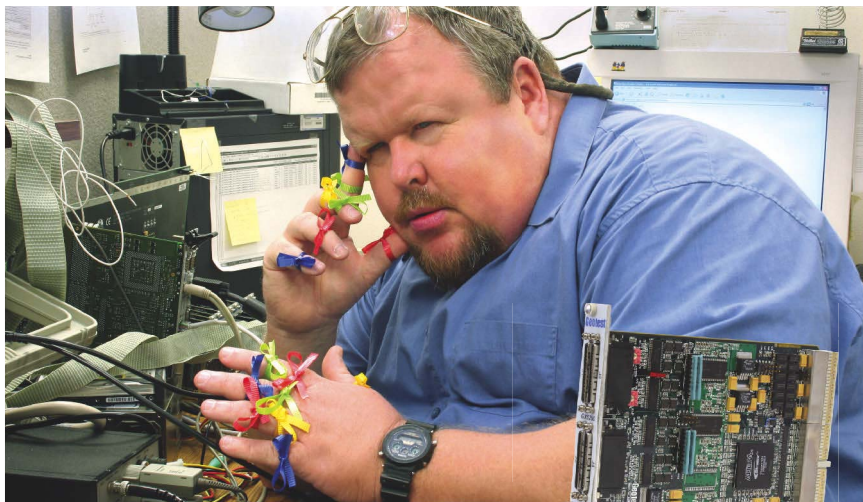
Using trigger signals to synchronize analog sensor operation with a boundary-scan clock allows PXI modules such as this power supply to extend scan test to encompass analog functions.
